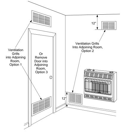
Figure 2 - Ventilation Air from Inside Building
